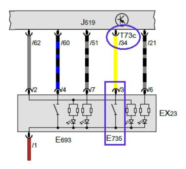
EX23 Switch module 1 in centre console E693 Start/Stop operation button
